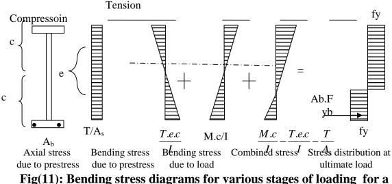
1): Bending stress diagrams for various stages of loading for prestressed steel beam.
