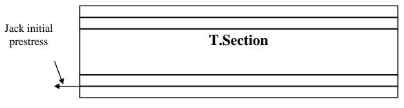
High strength plate( welded under stress)
