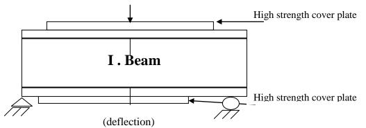
Fig(3): prestressing by deflecting A beam and attachingCover Plate
