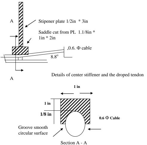
Fig(12): Detail of steel beam will straight and droped tendon
