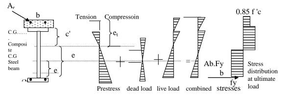
Fig (10): Bending stress diagrams for various stages of loading for a prestessesed composite steel beam
