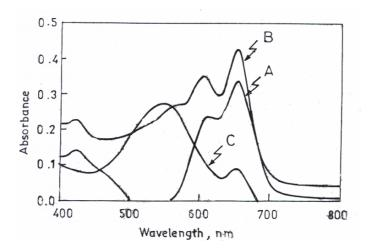
Fig.2:Absorption spectra of 10 µg mefenamic acid / 25 ml treated according to the recommended procedure and measured against (A) blank, (B) distilled water and (C) blank measured against distilled water.
