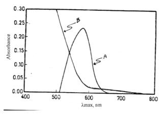
Fig 3: Absorption spectra of Zr(IV) – ECR (A) against reagent plank, (B) blank against distilled water.
