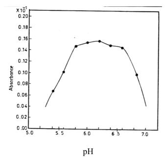
Fig 1: Effect of apparent pH on the absorption of Zr-ECR complex
