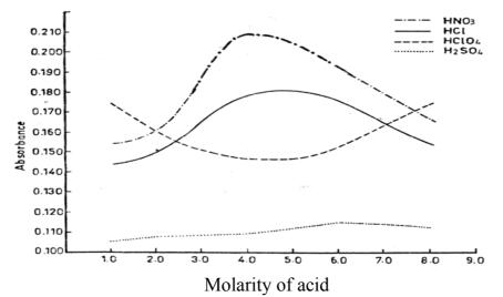
Fig 2: Extraction of Zr(IV) with TOPO in cyclohexane as a function of acid concentration
