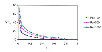
Fig.7 Variation of local Nusselt number along the bottom wall at AR=1 and R=1.5
