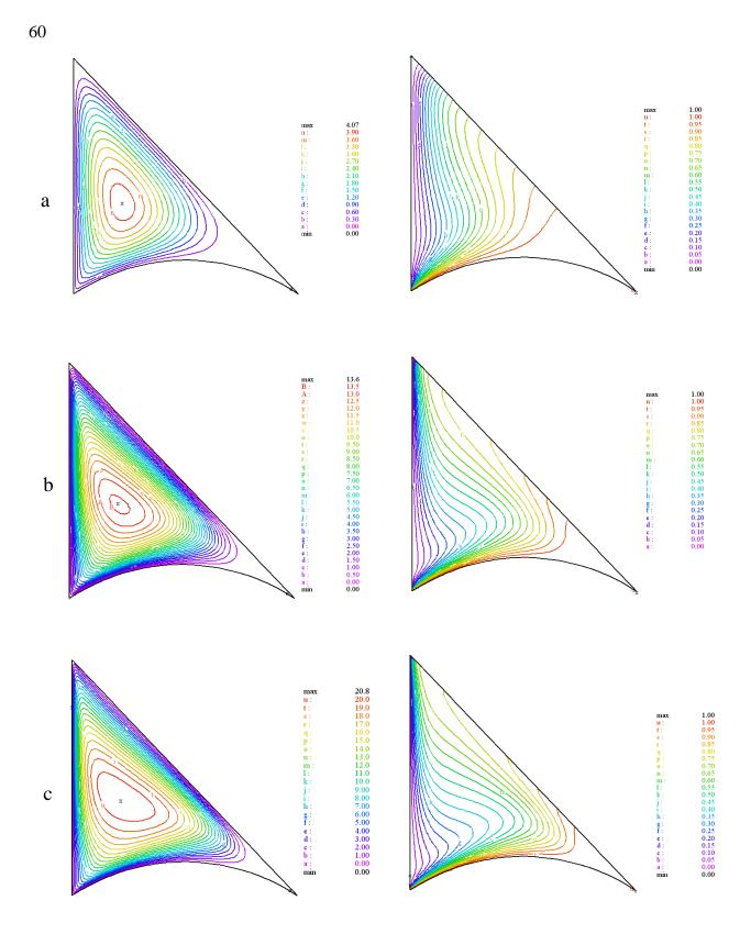
Fig.5 Streamlines (left) isotherms (right) at AR=1 and R=0.8 a) Ra=100 b) Ra=500 c) Ra=1000
