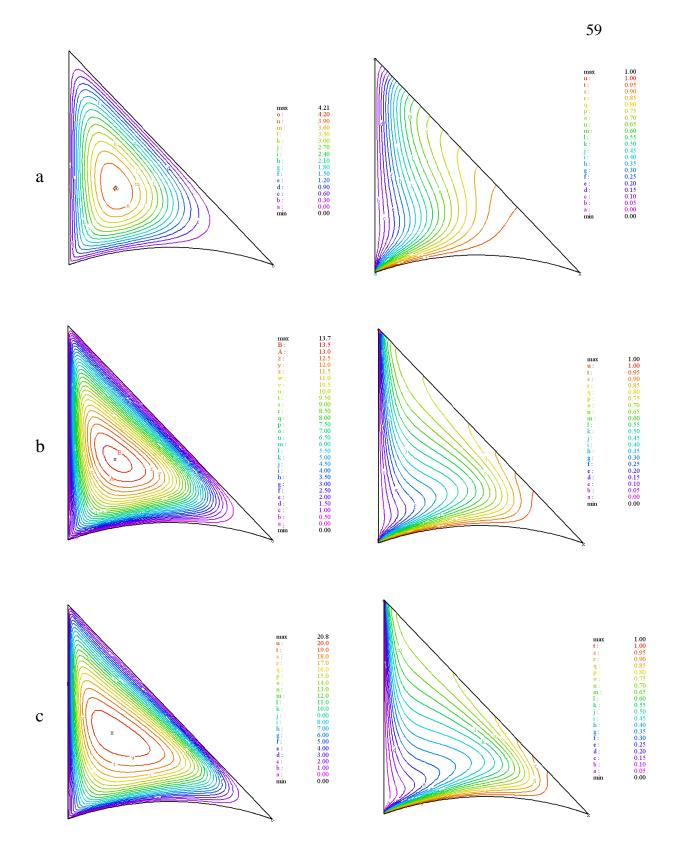
Fig.4 Streamlines (left) isotherms (right) at AR=1 and R=1.5 a) Ra=100 b) Ra=500 c) Ra=1000
