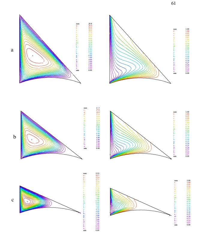
Fig.6 Streamlines (left) isotherms (right) at Ra=1000 and R=1.5 a) AR=1 b) AR=0.7 c) AR=0.4
