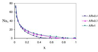
Fig.8 Variation of local Nusselt number along the bottom wall at Ra=1000 and R=1.5
