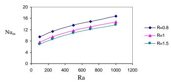
Fig.9 Variation of mean Nusselt number with Rayleigh number at AR=1 and different radius R .
