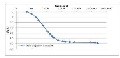
**Fig (7):** Collapse for soil model with 70% gypsum content using the new device for collapse test.(soaking stress=100kPa, soil density=17.3kN/m3).
