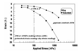
**Fig.(10):** Double odometer collapse test proposed by for (Jennings, J.E. and Knight, K. 1975) for the used soil with gypsum content=30%.
