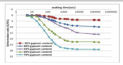
Fig (8): Results of laboratory test on model samples to semulate the collapsibility of gypseous soil with different gypsum content using MCT device.(stress level=100kPa, soil density=17.3kN/m<sup>3</sup>).
