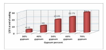
**Fig (9):** Deformation ratio S/B% for soils with different gypsum content tested by the MCT device.(stress level=100kPa, soil density=17.3kN/m<sup>3</sup>).
