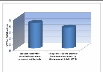
**Fig (11):** Collapse measuring using the MCT device proposed in this study, compared with that measured using the ordinary double oedometer collapse test, proposed by Jenings, J.E. and Knight, K. 1975) in measuring collapsibility of gypseous soil.(G.C=30%, soaking stress=100kPa).
