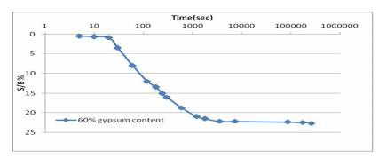
**Fig (6):** Collapse for soil model with 60% gypsum content using the new device for collapse test.(soaking stress=100kPa, soil density=17.3kN/m3).
