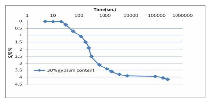
**Fig (3):** Collapse for soil with 30% gypsum content using the new device for collapse test.(soaking stress=100kPa, soil density=17.3kN/m3).
