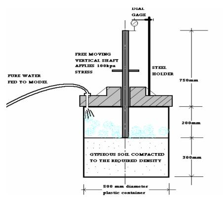
Fig. (2-b): parts and mechanism of (MCT) proposed in this study.
