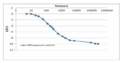
**Fig (4):** Collapse for soil with 40% gypsum content using the new device for collapse test.(soaking stress=100kPa, soil density=17.3kN/m3).
