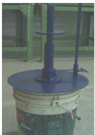
Fig.(2-c): Setting of MCT instrument over the model test sample containing gypsiferous soil, for laboratory model collapse test.
