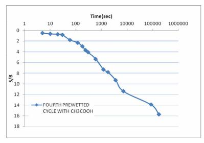
**Fig.(5):** soaking time vs. S/B% for gypseous soil model wetted four cycles by CH3COOH acid. .(G.C=70%, soil density=17.3kN/m<sup>3</sup>).
