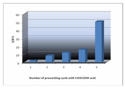
**Fig(8):** Final collapse settlement in terms of S/B%, against number of cycles of wetting gypseous soil by CH3COOH acid.(G.C=70%, soil density=17.3kN/m<sup>3</sup>).
