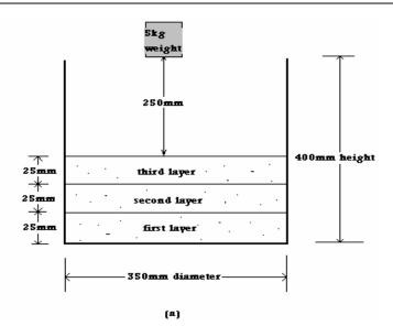
Fig.(1-a): Soil preparation and density control for laboratory model sample.
