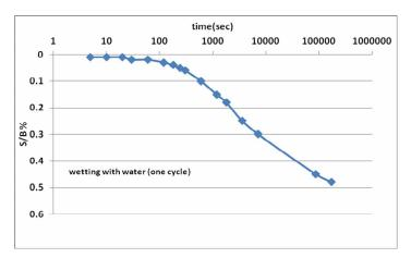
**Fig.(2-b):** Soaking time vs. S/B% for gypseous soil model wetted by water.(G.C=70%, soil density=18.4kN/m<sup>3</sup>).
