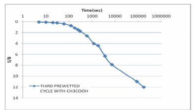
**Fig.(4):** Soaking time vs. S/B% for gypseous soil model wetted three cycles by CH<sub>3</sub>COOH acid.(G.C=70%, soil density=17.3kN/m<sup>3</sup>).
