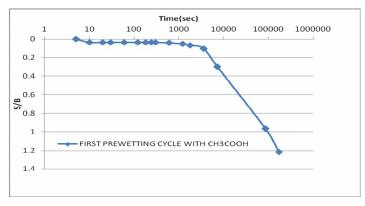
**Fig.(2-a):** Soaking time vs. S/B% for gypseous soil model prewetted by CH<sub>3</sub>COOH acid.(G.C=70%, soil density=17.3kN/m<sup>3</sup>).
