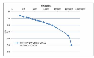
**Fig.(6):** soaking time vs. S/B% for gypseous soil model wetted five cycles by CH3COOH acid. .(G.C=70%, soil density=17.3kN/m<sup>3</sup>).
