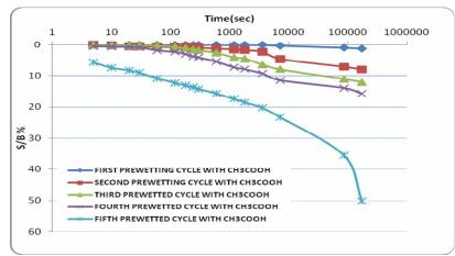
Fig.(7): Effect of wetting cycles by CH3COOH acid on the collapsibility of gypseous soil.  $(G.C=70\%, soil density=17.3 kN/m^3)$ .
