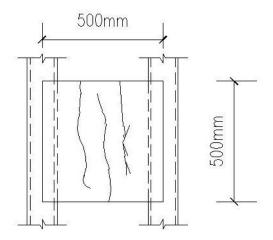
**Fig.(5):**The crack pattern (S<sub>2</sub>).
