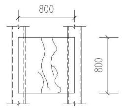
**Fig.(7):**The crack pattern (S<sub>4</sub>).
