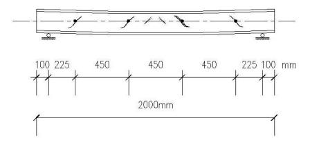
Fig. (4):Bolt position and the cracks pattern.
