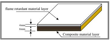
Fig (2): Specimen of thermal erosion test.
