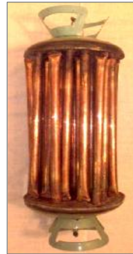
Figure(2): Both parts of generator after combined together
