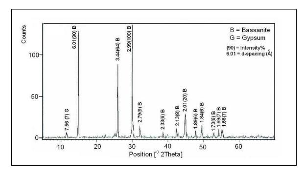
Fig. 5: X-Ray Diffraction Peaks for Dental Stone.
