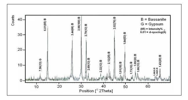
Fig. 3: X-Ray Diffraction Peaks for Rasheed Plaster.
