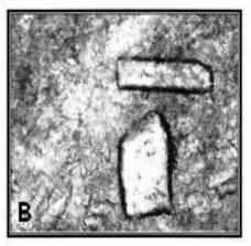
Plate (2) : Rasheed Plaster. A- Before Compression .. Crystals subrounded, with ill-defined edges of the type  $\beta$ - hehihydrate . B- After Compression. Prismatic monoclinic crystals, with sharp edges of the type  $\alpha$ - hemihydrate.
