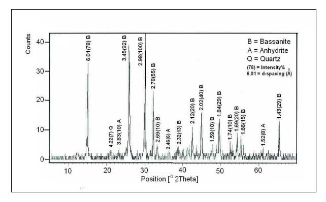
Fig. 4: X-Ray Diffraction Peaks for Madae'n Plaster.
