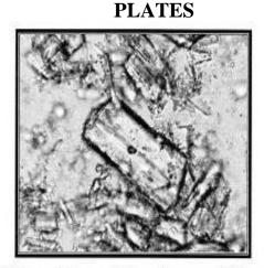
Plate (1):Dental Stone. Prismatic monoclinic crystals of Bassanite of the type a- hemihydrate.
