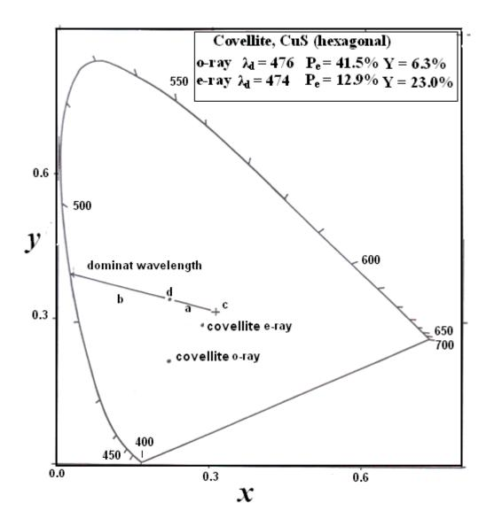
Fig. 3:The CIE (1931) Chromaticity Diagram (Judd, 1952). Derivation of Helmholtz Colour Coordinates  $\lambda_d$  and  $P_e$  for Mineral Plotted at Point (d) is as Follow:
