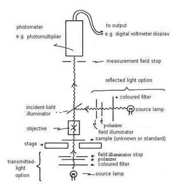
Fig. 5: Simplified Diagram of Essential Components of Micro-Photometer.
