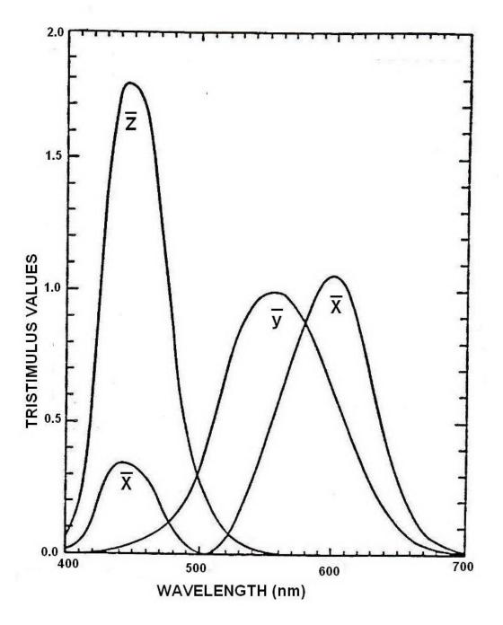
Fig.1: Spectral Curves of the Tristimulus Values of the Spectrum Colours. These Curves form the Basis of the CIE (1931) Colour System and Correspond to the Spectral Sensitivity of the CIE Standard Eye. CIE= is Commission Internationale d'Eclairage.
