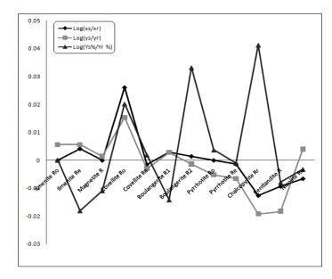
Fig. 6: Correlation Sketch Diagram (accuracy %) between Obtained Colour Values of this Study  $(x_s, y_s \text{ and } Y_s\%)$ and Corresponding Reference Values  $(x_r, y_r \text{ and } Y_r\%)$ .
