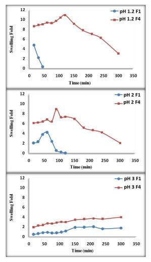
Figure 6: Effect of forming semi-IPN on the swelling fold of chitosan only formula (F1) and chitosan / PVP formula (F4) at 37°C in different pH
