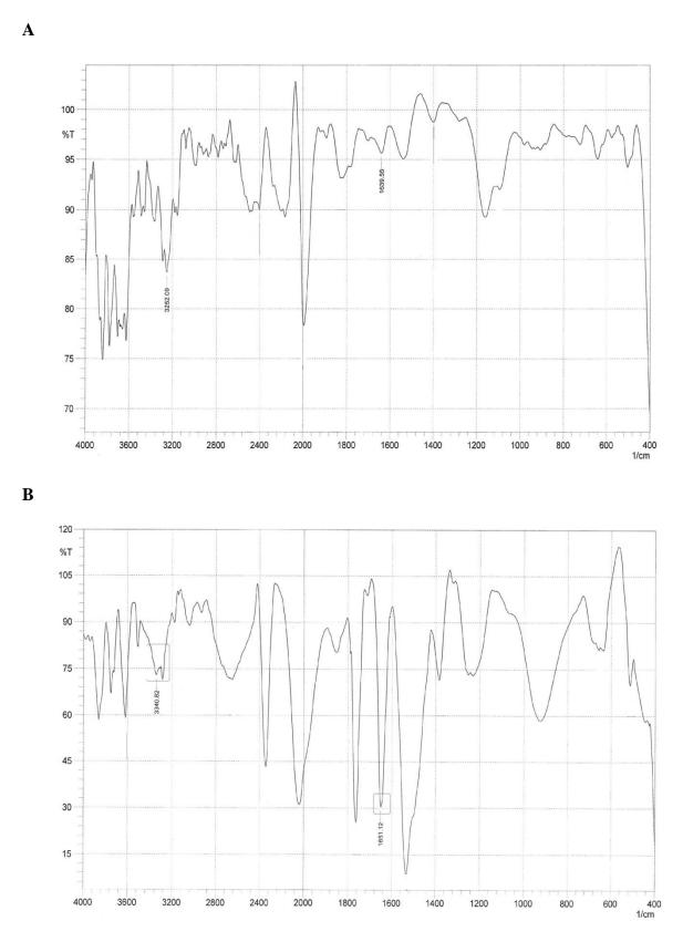
Figure 2: FT-IR spectrum of (A) non- crosslinked chitosan polymer (B) crosslinked chitosan polymer with GA
