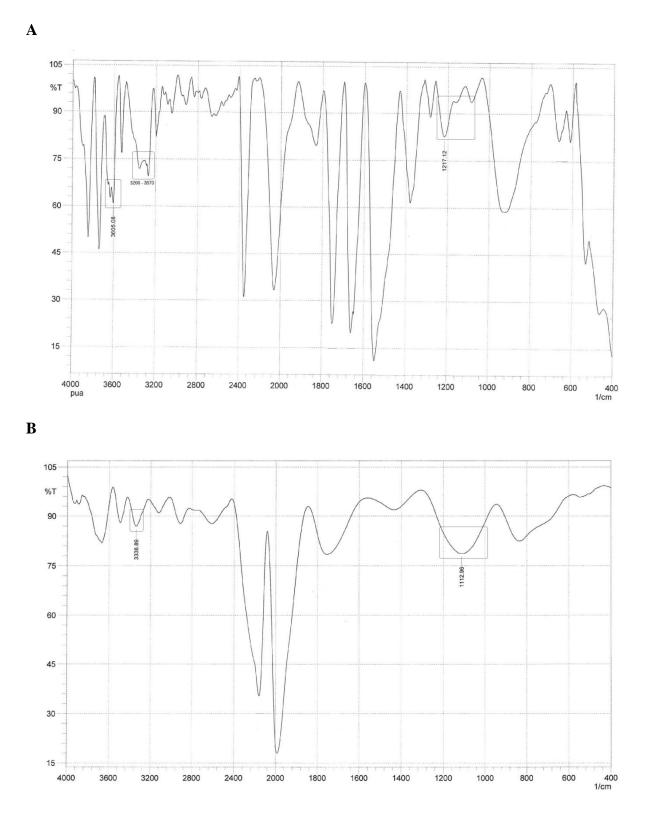
Figure 3: FT-IR spectrum of (A) non-crosslinked PVA (B) crosslinked PVA with GA
