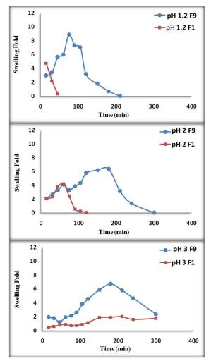
Figure 7: Effect of forming semi-IPN on the swelling fold of chitosan only formula (F1) and chitosan / PVP formula (F9) at 37°C in different pH
