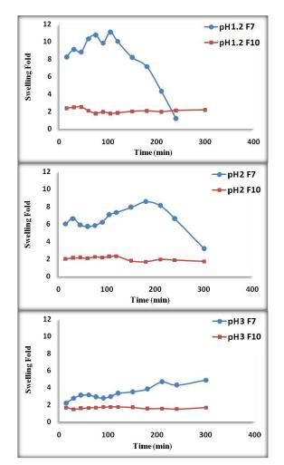
Figure 11:Effect of using PVA on the swelling fold of networks of chitosan/PVP (formula **F7**) and chitosan/PVA (formula **F10**) at 37°C in different pH
