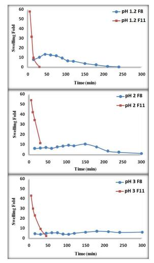
Figure 5: Effect of freeze-drying on the swelling fold of freeze-dried formula (**F11**) and air-dried formula (**F8**) at 37°C in different pH
