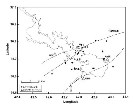
Fig. 2: Seismicity Map of Mosul's Reservoir for the Monitoring Period January to 20<sup>th</sup> July 1990.
