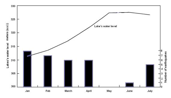
Fig.4: The Relationship between the Lake's Water Level and the Number of the Located Earthquakes, During the Monitoring Period.
