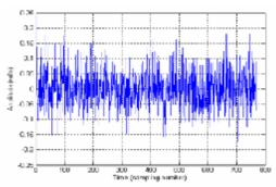
Figure (8)Fig. (8) Wave form for OFDM signal in time domain
