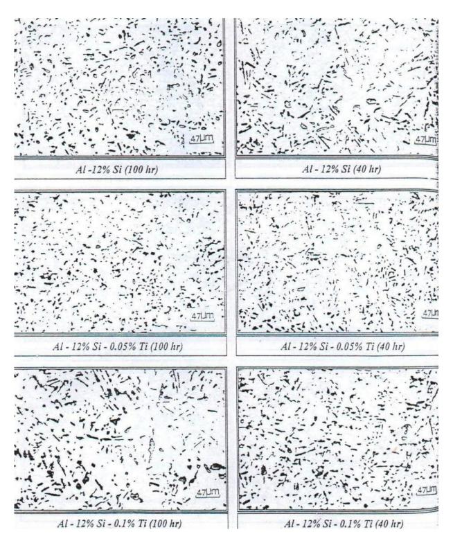
Fig.(4): Microstructure of Homogenized Alloys with (40 , 100 )hrs. at 525  $^\circ\mathrm{C}$
