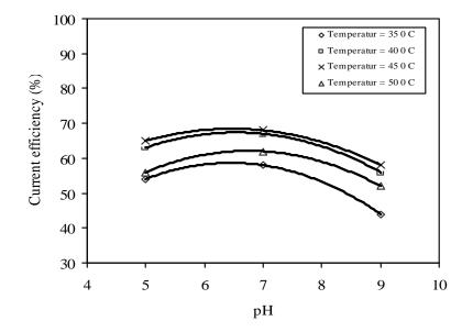
**Fig. (9):** Variation of Current Efficiency with pH as a function of Temperature at Anode Current Density = 25 Amp/dm2
