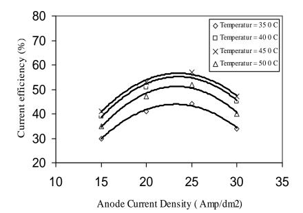
**Fig. (4):** Variation of Current Efficiency with Anode Current Density as a function
