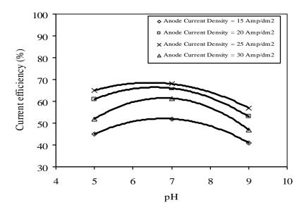
Fig.(8): Variation of Current Efficiency with pH as a function
