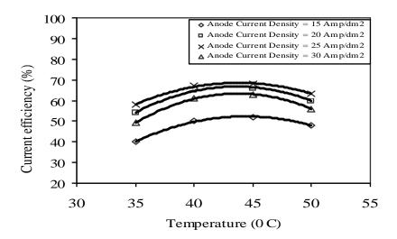
Fig. (6): Variation of Current Efficiency with Temperature as a function of Anode
