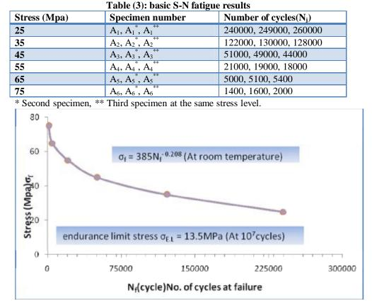
Figure (2a): basic S-N curve for 1100 Al alloy
