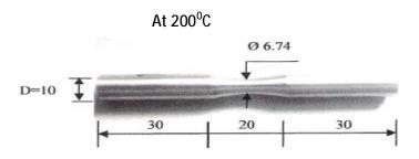
Figure (2): geometry of fatigue creep interaction specimens; dimensions
