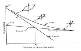
Figure (3) Strain-Life Curve [9]
