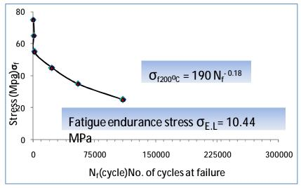
Figure (2b): The S-N curve at 200° C
