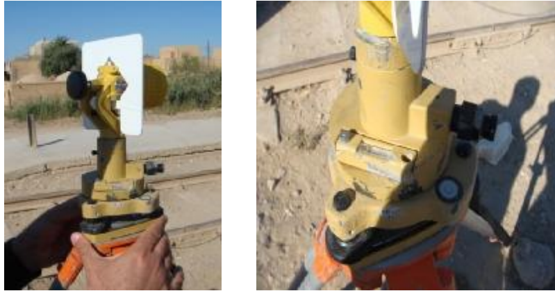
Figure (7): illustrate the adjustment and centering of prism rods
