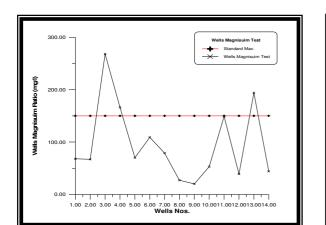
Figure (13) Magnesium results test with standards
