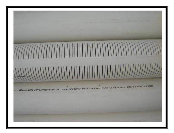
Figure (8) Screen filter pipes making in a special factory
