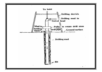
Figure (4) Deep well construction using by Hydraulic-rotary Method
