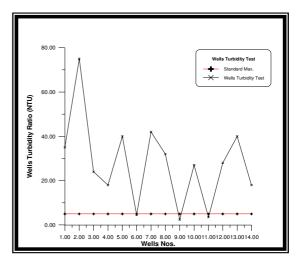
Figure (12) Turbidity results test with standards
