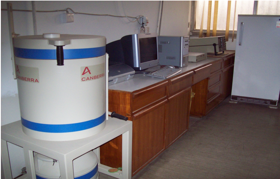
Figure (2): A gamma- ray spectrometry system
