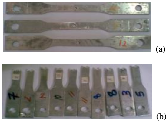
Figure (2) Tensile test specimens (a-before test, b-after test).
