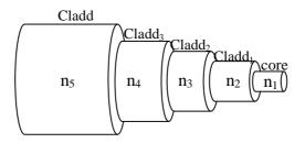
Figure (2): five layer cylindrical dielectric structure
