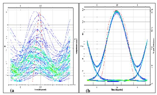
Figure(6): Illustrate the eye diagram of RZ format transmit over optical transmission system with standard single mode fiber length of 50km . a: without using DCF b: with using proposed DCF at length of 1km.
