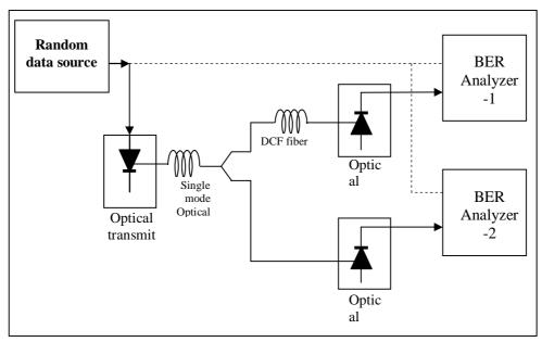
Figure(5): The experiment setup of optical fiber communication system with using DCF.
