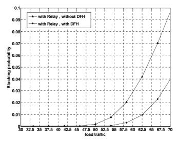
Figure (7) The relationship between  $P_B$  and load traffic when K = 13, number of calls =25 per hour, average calling time = 2 minute
