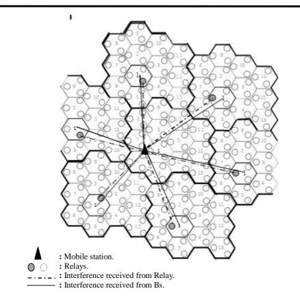
Figure (2) The interference sources (BS, Relays) when the cluster size is equal to 13.
