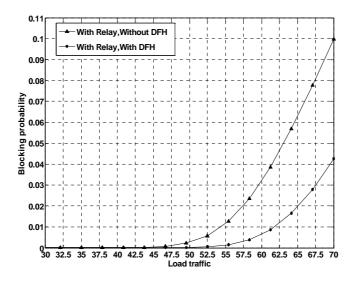
Figure (8) The relationship between  $P_B$  and load traffic when K = 7, number of calls =35 per hour, average calling time = 1 minute
