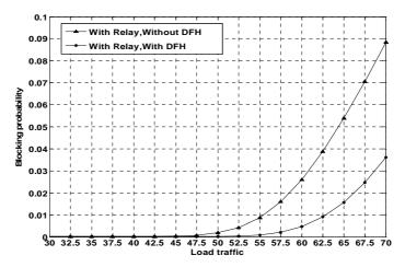
Figure (5) The relationship between  $P_B$  and load traffic when K = 13, number of calls = 15 per hour, average calling time = 2 minute
