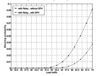
Figure (9) the relationship between  $P_B$  and load traffic when K = 13, number of calls =35 per hour, average calling time = 1 minute
