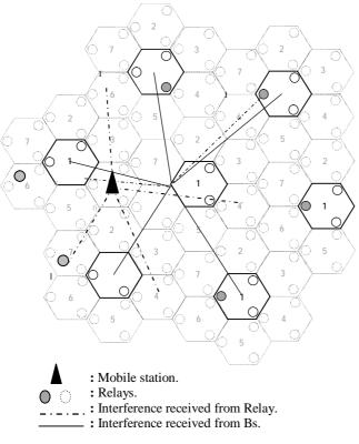
Figure (1) The interference sources (BS ,Relays) when the cluster size is equal to7
