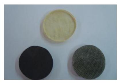
Figure (2) Samples of research that coincide (ASTM-D150),(1)Pure Epoxy , (2)Epoxy +Al powder,(3)Epoxy +Al fiber
