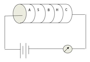
Figure (1) Schematic diagram of Lees Disk
