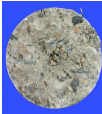
b- Large Failure cone d_b=10\text{mm} , h_{ef}=37.5\text{mm} v_f=1.2\% , l_f=32\text{mm}
