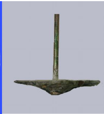
a -Concrete Failure cone d_b=8\text{mm} , v_f=0\% , h_{ef}=25\text{mm}
