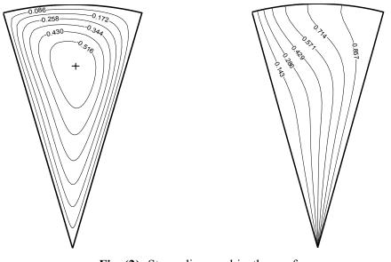
Fig. (2): Streamlines and isotherms for  $Ra^*=100, \Phi=30^{\circ}$ .
