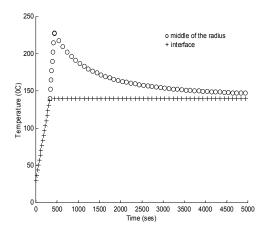
Fig.( 4): Temperature-time history at the interface and the middle of the sample (B).
