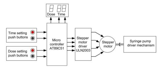
Figure(3) : The block diagram and connection of (ULN2003) as stepper motor driver of Drug Delivery System.
