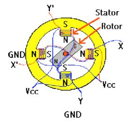
Figure (1): diagram of a stepper motor coils connection.
