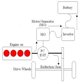
Figure 7 Engine/charge mode.
