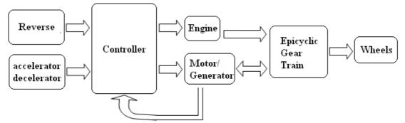
Figure 15 Functional interrelations between subsystems.
