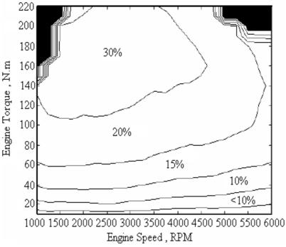
Figure 1 Typical engine efficiency map [1].
