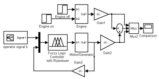
Figure 16 Operational block diagram of the speed control system.
