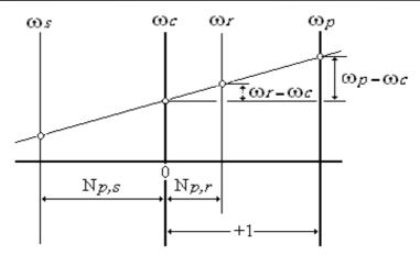
Figure 3 Nomograph for the basic epicyclic gear train [8].
