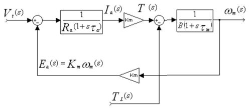
Figure 13 Block diagram representation of a DC motor.
