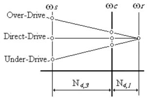
Figure 11 Nomograph for the power mode of the new hybrid transmission.
