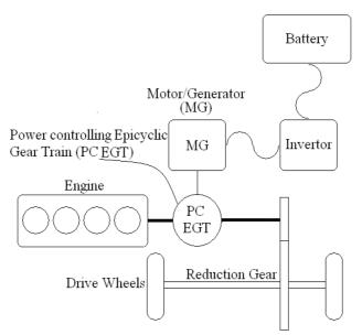
Figure 5 Block diagram of the new hybrid system.
