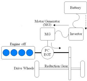
Figure 6 Electric motor mode.
