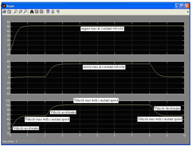
Figure 19 Simulation results for acceleration, deceleration or cruising of the car.
