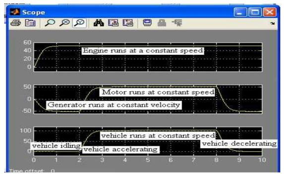
Figure 22 Simulation results for idling, acceleration, deceleration or cruising of the car.
