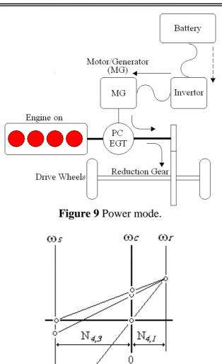
Figure 10 Nomograph for the engine and engine-charge modes of the new hybrid transmission.
