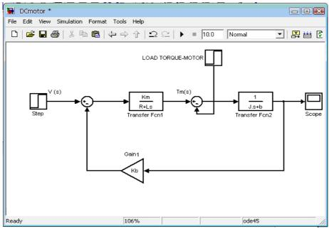
Figure 14 Block diagram representation of a DC motor in SIMULINK.
