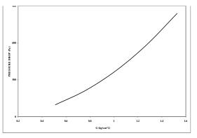
Fig. (13) Pressure drop with respect of mass flow rate per cross section area in case2.
