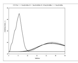
Fig. (10) Change in temperatures between inlet and outlet air in case1
