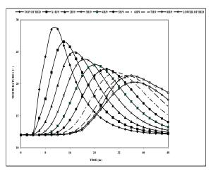
Fig. (5) Temperature distribution in the rock bed during 48 hrs, for  $D_R=0.05m$ .
