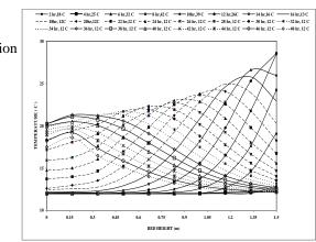
Fig. (2) Temperature distribution in the rock bed during 48 hrs, for  $D_R=0.01m$ .
