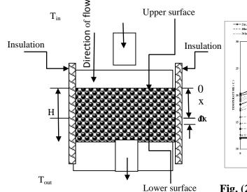
Fig. (1) Schematic of rock bed thermal storage
