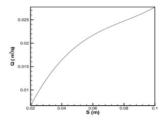
Figure 9: The relation between induced flow rate with the width of the channel.
