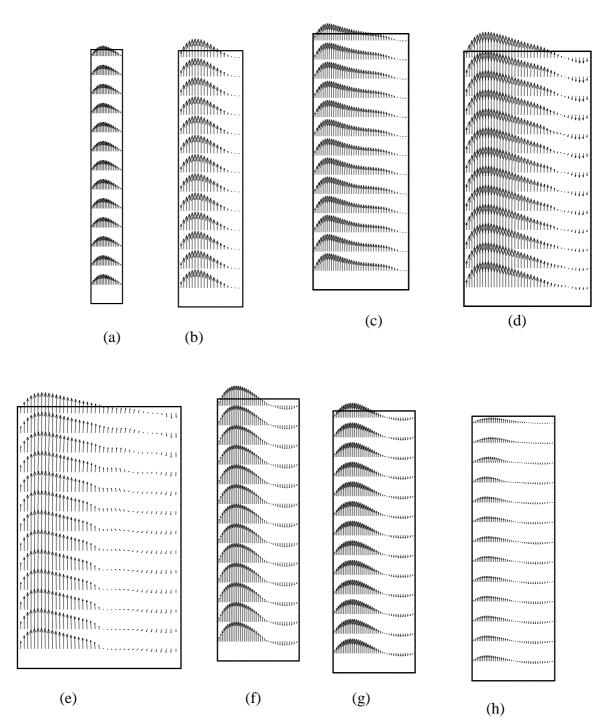
Figure 5. Velocity vector within the channel at  $\Delta T = 30$  for (a) A=20, (b) A=10, (c) A=6.6, (d) A=5, (e) A=4, and  $\Delta T = 30,20$  and 10 for A= 8 in f, g and h respectively.
