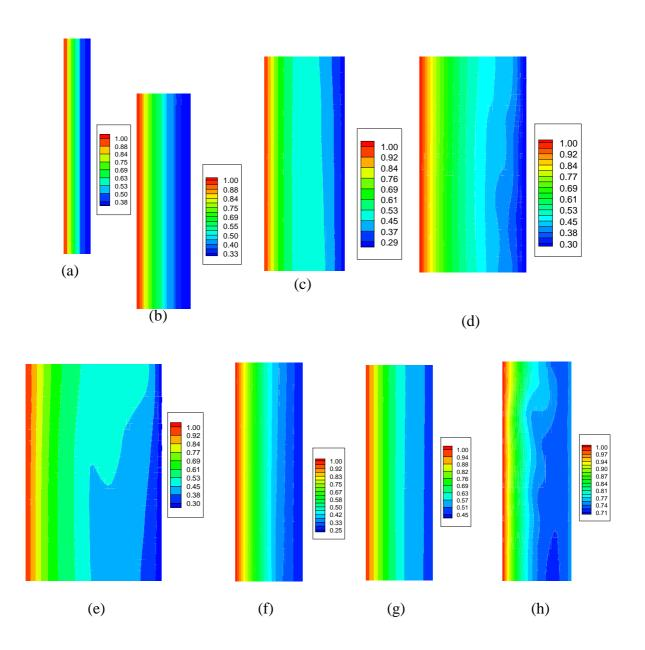
Figure 4. Non-dimensional temperature contour ( $\theta$ ) at  $\Delta T = 30$  for (a) A=20, (b) A=10, (c) A=6.6, (d) A=5, (e) A=4, and  $\Delta T = 30,20$  and 10 for A= 8 in f, g and h
