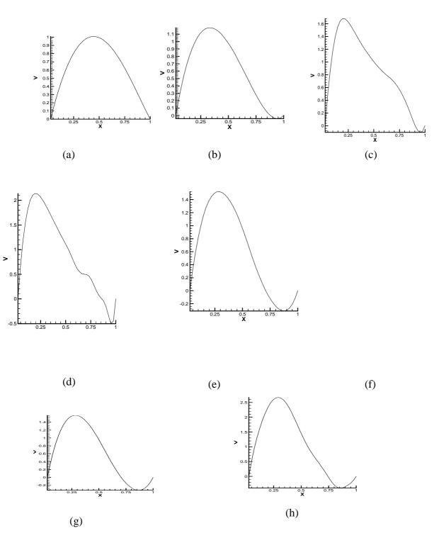
Figure 6. Non-dimensional axial velocity component at exit (V) at  $\Delta T = 30$  for (a) A=20, (b) A=10, (c) A=6.6, (d) A=5, (e) A=4, and  $\Delta T = 30$ ,20 and 10 for f, g and h respectively.
