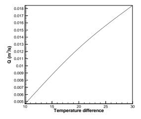
Figure8: The relation between induced flow rate with the temperature difference of the walls.
