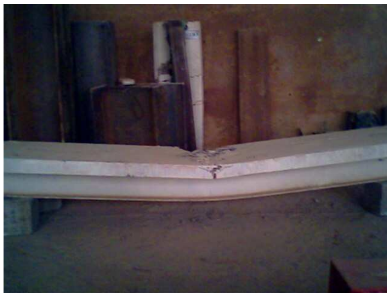
Figure (4): Beam CB0 at Failure
