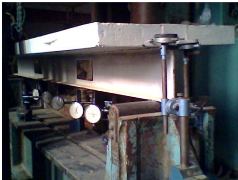
Figure (3): Typical Setting for Composite Beams before Testing
