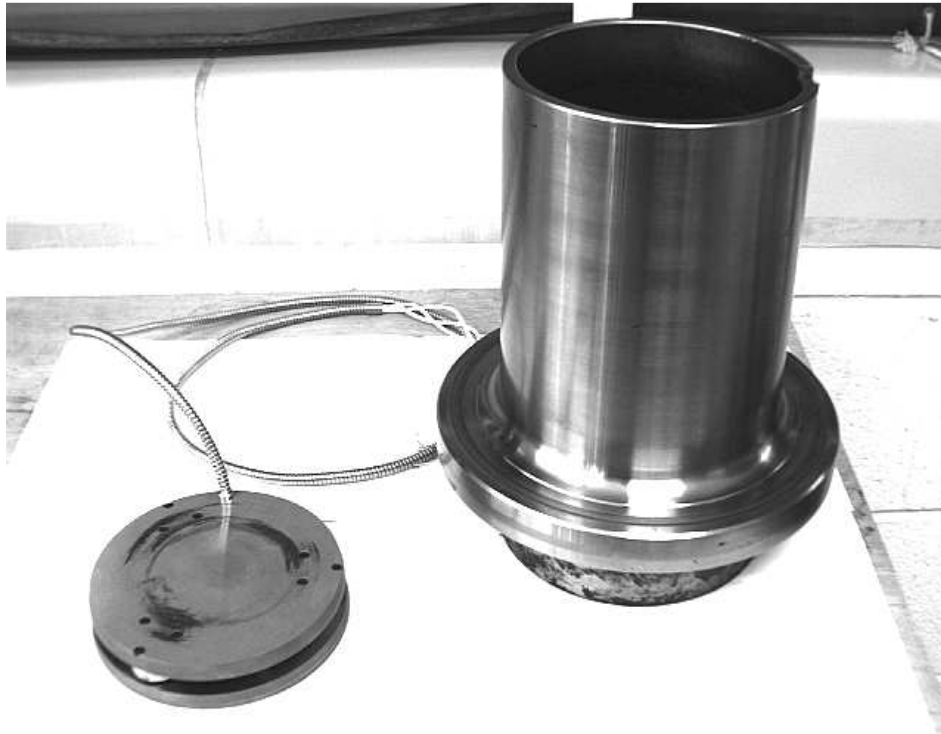
Figure 8 The Pressure Distribution Analyzer (PDA) Shear Plate Used in the SGC Compaction Mold
