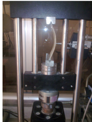
(b) After Buckling
