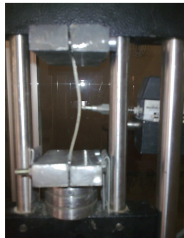
(b) After Buckling
