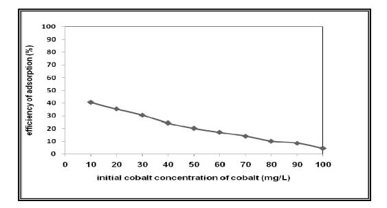
Figure (1) Effect of Initial Co (II) Concentration of Efficiency Of Adsorption% of Cobalt
