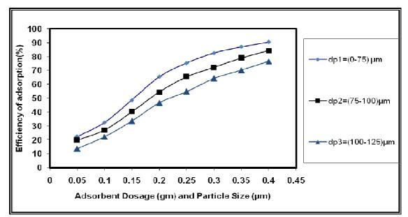
Figure (3) Effect of Adsorbent Dosage and Adsorbent Particle Size Efficiency of Adsorption% of Co (Initial cobalt (II) concentration = 10 mg/L, pH =13, contact time = 30 min, and shaking= 150rpm)
