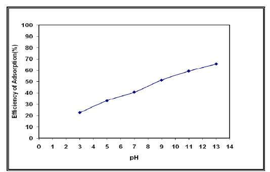
Figure (2) Effect of pH on Efficiency of Adsorption% of Co (Initial cobalt (II) concentration =10 mg/L, adsorbent dose= 0.2 gm/100 mL, adsorbent particle size =  $(0-75)\mu$ m, contact time =30 min, and shaking rate = 150 rpm)
