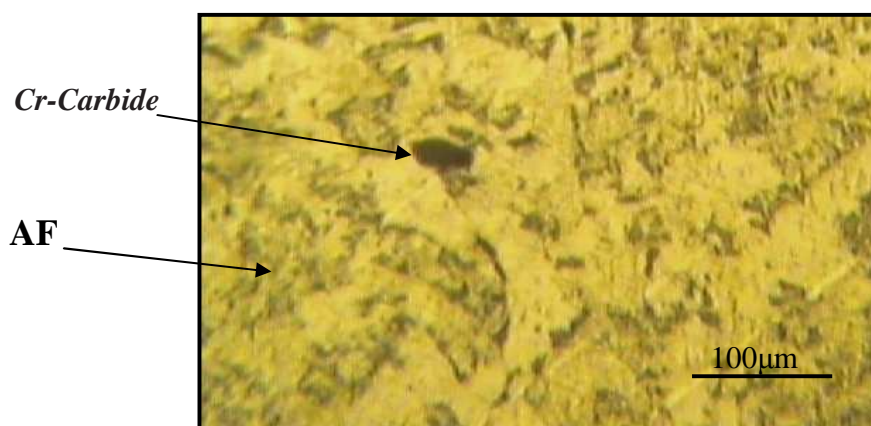
Figure2. Optical microscopy of the weldment when F71-EM12K filler metal was used.
