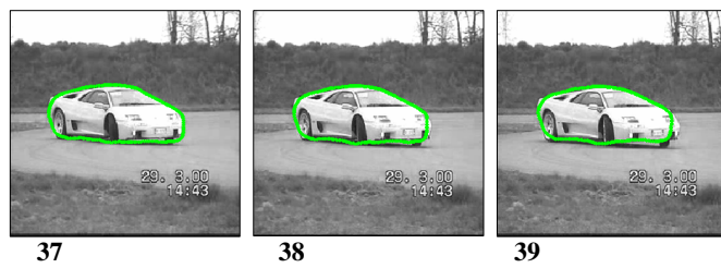
Figure (12): The tracking operation of the rally car during its rotation in the scene.
