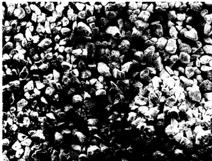
Figure 6 Scanning electron micrograph of the prepared potassium fluorosilicate ( EHT=20.00Kv , WD=9.0mm , Signal=SE1 )
