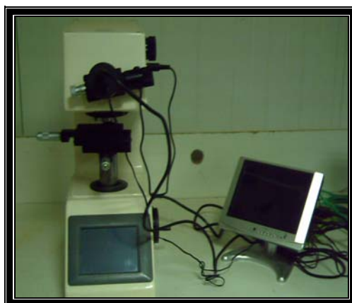
Figure 3 The digital micro Vickers hardness tester was used to conduct the test with a load of 100g for 20 sec.
