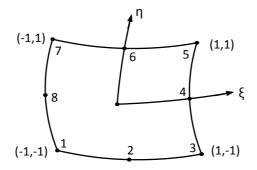
Figure 4 Eight-node quadrilateral isoparametric element.
