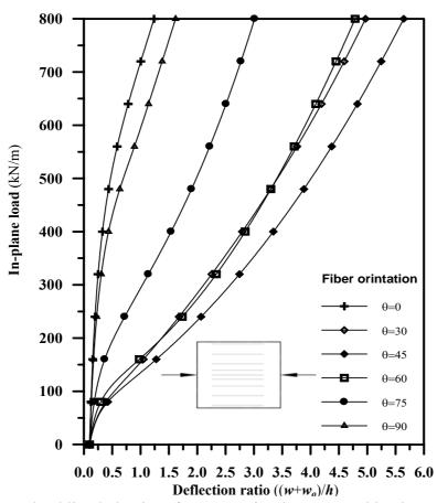
Figure 8 Post-buckling behavior of a square simply supported laminated composite plate with variable fiber spacing with various fiber orientations
