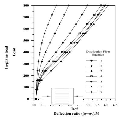
**Figure 7** Post-buckling behavior of a square simply supported laminated composite plate with variable fiber spacing under in-plane loading at *x*-direction
