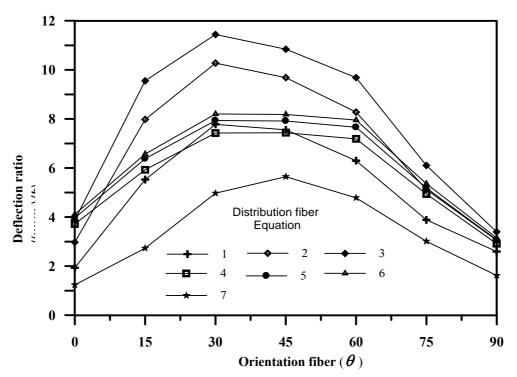
Figure 9 Deflection-orientation fiber curve of composite laminated plate under in-plane compression load at *x*-direction
