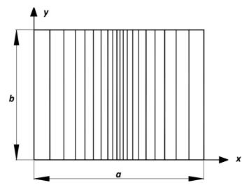
Figure 3 rectangular composite plates with variable fiber spacing.
