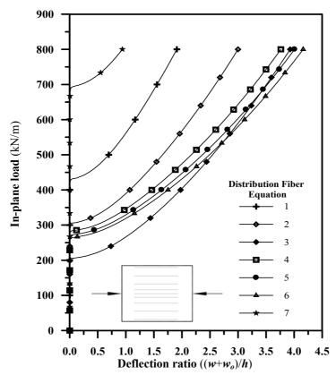
Figure 5 Post-buckling behavior of a square simply supported laminated composite plate with variable fiber spacing under uniaxial compression load *x*-direction.
