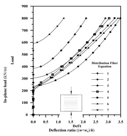
**Figure 6** Post-buckling behavior of a square simply supported laminated composite plate with variable fiber spacing under uniaxial compression load *y*-direction.
