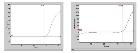
Figure 2: Showing two positive cases with two different (Ct)s (28.3 and 33.9 ) which indicates different levels of viral genome .
