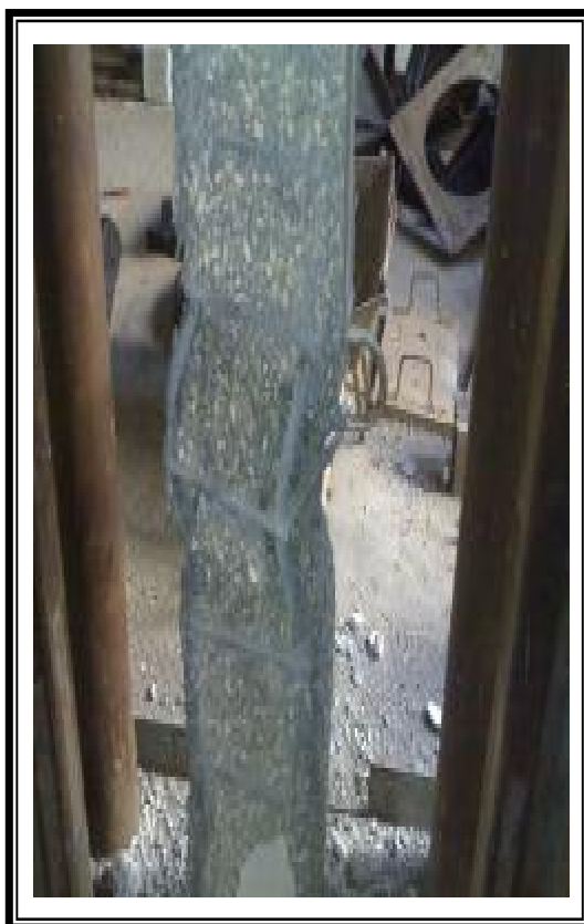
Figure (7) Failure Mode of Column A_1B_2C_1 Figure (8) Failure Mode of Column A_1B_2C_2
