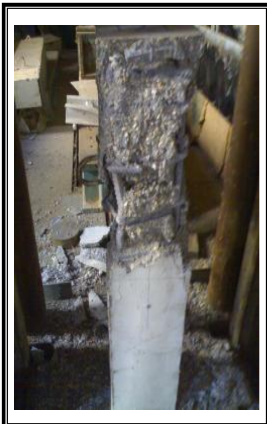
Figure (7) Failure Mode of Column A_1B_2C_1 Figure (8) Failure Mode of Column A_1B_2C_2
