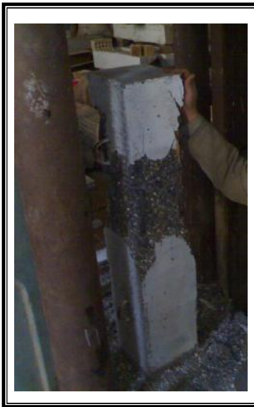
Figure (5) Failure Mode of Column A_1B_1C_1 Figure (6) Failure Mode of Column A_1B_1C_2
