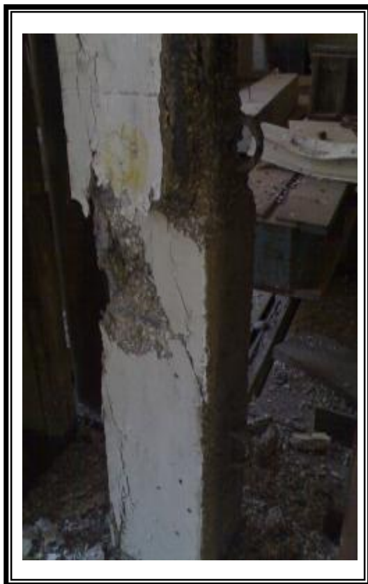
Figure (5) Failure Mode of Column A_1B_1C_1 Figure (6) Failure Mode of Column A_1B_1C_2
