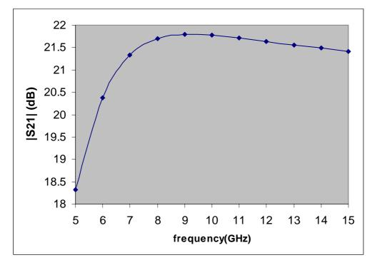
Fig. 3 : TIA gain versus frequency.
