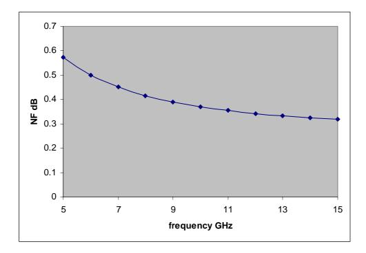
Fig. 7: Minimum noise figure before applying noise at TIA input.
