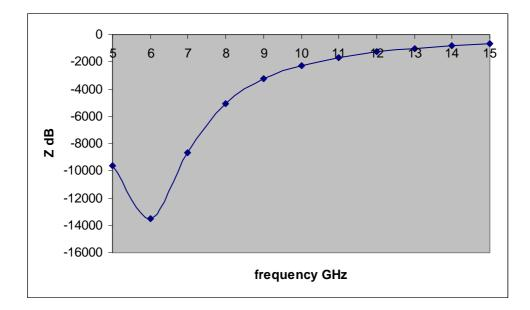
Fig. 6: TIA input impedance (real part) which confirm TIA circuit stability factor.
