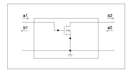
Fig.1: A transistor two port network.
