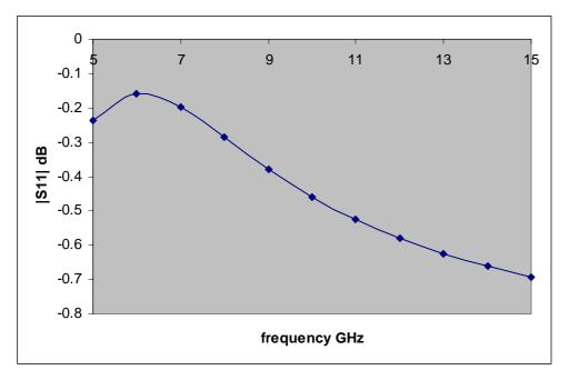
Fig. 4: Reflected signal from TIA input versus frequency.
