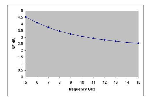
Fig. 9: Minimum noise figure after applying noise at TIA input.
