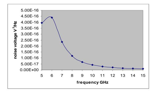
Fig. 8: Noise voltage before applying noise at TIA input.
