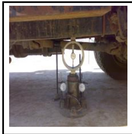
b. Closed view of Plate Load Test
