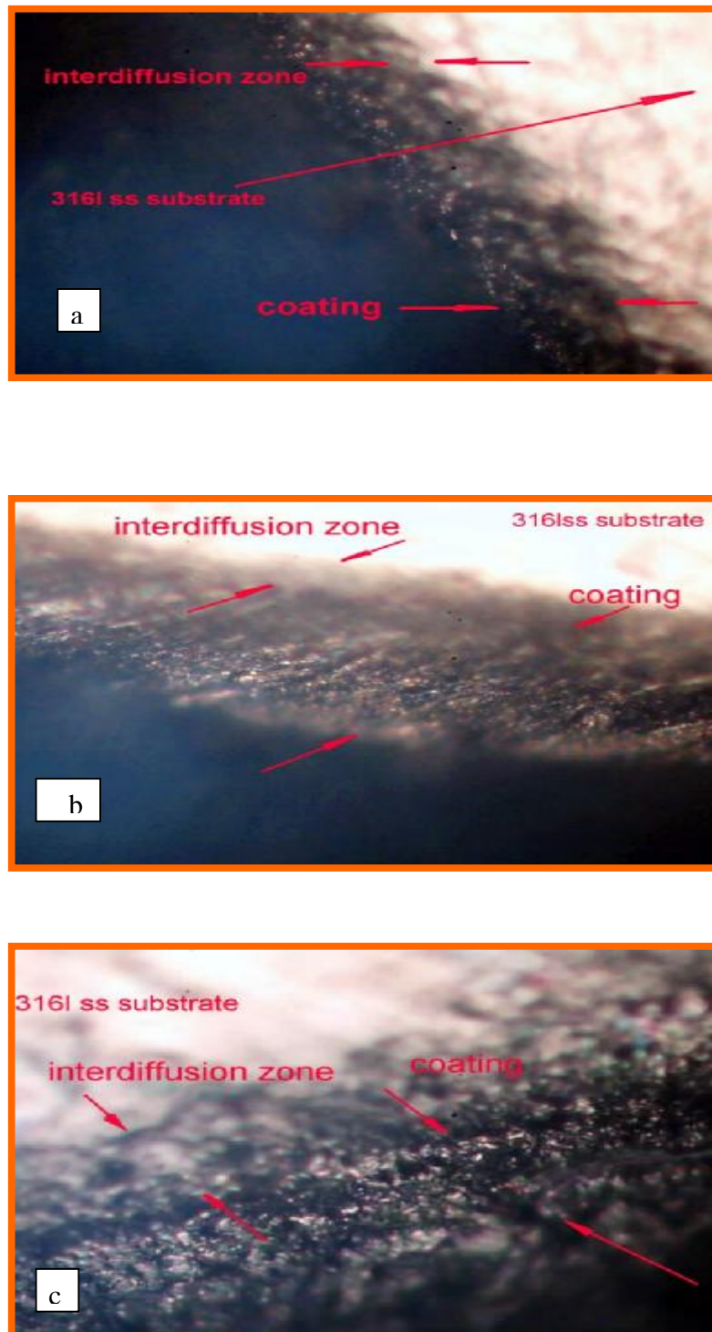
Figure (9) LOM images of 316Lst.st alloy siliconized at 950°C for 4hr a- for sample coated with pack activated by 5% NH 4 Cl b- for sample coated with pack activated by 7% NH 4 Cl c- for sample coated with pack activated by 10% NH 4 Cl
