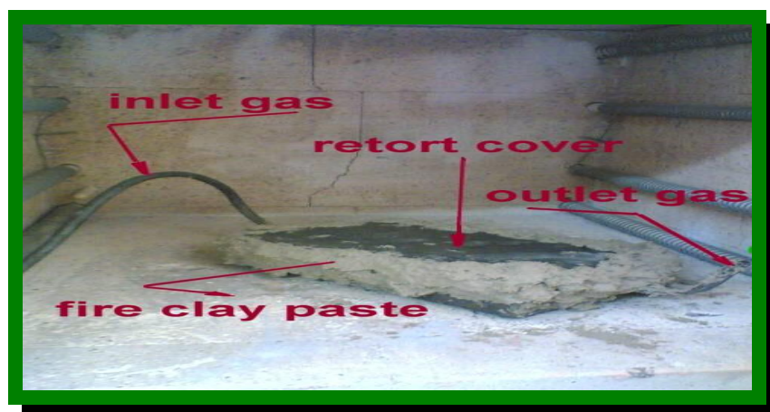
Figure (3) retort plugged with fire clay paste inside uniform heated zone of furnace
