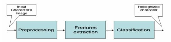
(Figure-1) The typical OCR block diagram
