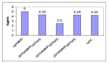
Figure (5) Energy gap values of PMMA/PC blends
