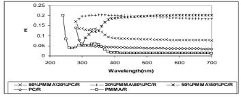
Figure (2) Optical reflection spectra of PMMA/PC blends
