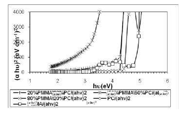
Figure (4) ( $\alpha hv$ )<sup>2</sup> versus (hv) of PMMA/PC blends
