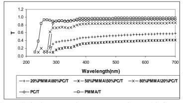
Figure (3) Optical transmittance spectra of PMMA/PC blends
