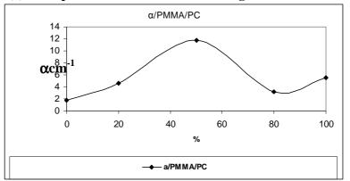
Figure (7) The absorption coefficient versus concentration ratio for binary blends (at  $\lambda_{\text{cut off}}$ ).
