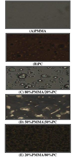
(E) 20%PMMA/80%PC Figure (16) Optical micrographs of PMMA/PC; show the immiscibility or phase separations at different concentration(X10).
