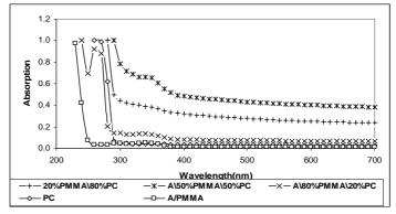
Figure (1) UV/Visible absorption spectroscopy of PMMA/PC blends
