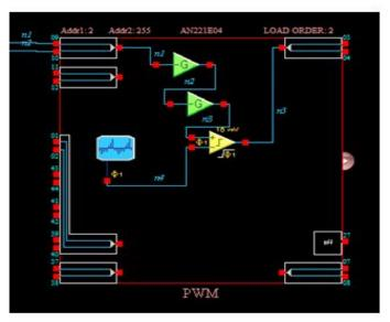
Fig. (5): PWM using FPAA technology. **2.3. Self-tuning of PID controller**
