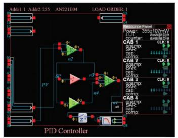
Fig.(4): Implementation of the PID Controller in FPAA.
