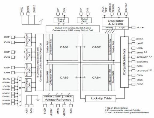
Fig. (3): Block diagram of AN221E04 FPAA.
