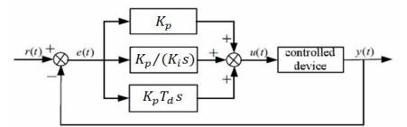
Fig. (2): PID Controlled system
