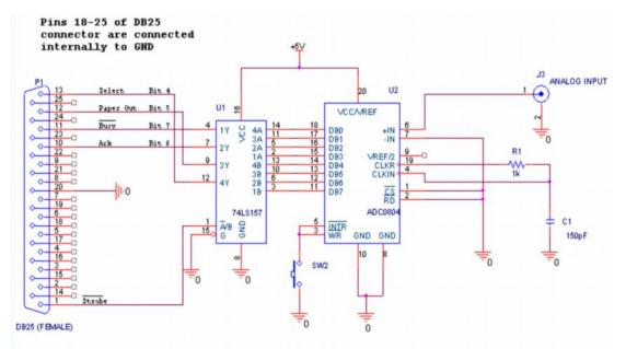
Fig. (8): Hardware circuit connecting ADC0804 to a PC through parallel port.
