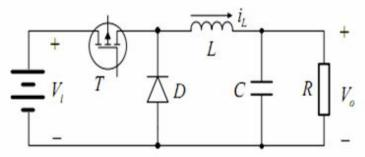
Fig. (7): Buck converter topology.
