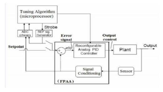
Fig. (6): Self-tuning PID controller architecture
