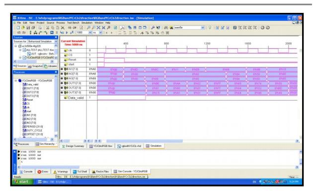
Figure 4: The YCbCr to RGB waveform conversion
