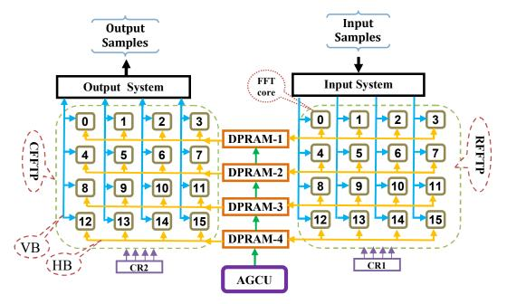
Figure (4) 2D FFT system architecture
