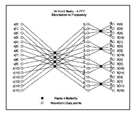
Figure (1) 16-point Radix-4 DIF-FFT signal flow diagram
