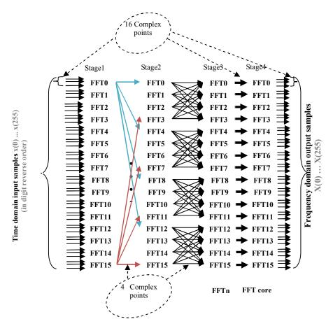
Figure (3) Flow graph of reconfigurable 1D FFT
