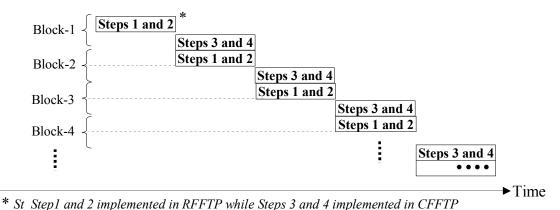
Figure (7) Overlapping in implementing 2D FFT algorithm in proposed system
